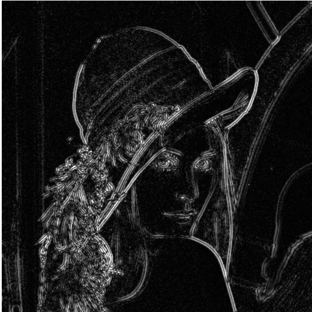
Laplacian of Gaussian filtering
