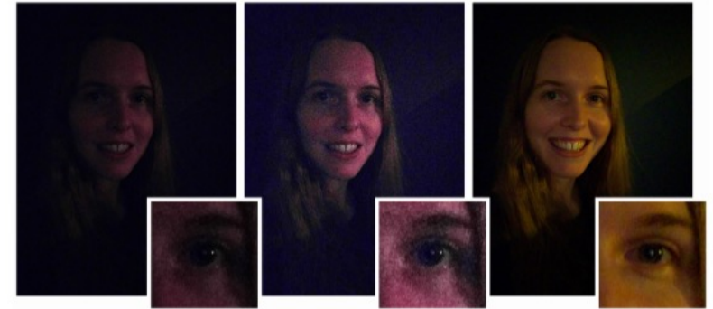
Figure 1: A comparison of a conventional camera pipeline (left, middle) and our burst photography pipeline (right) running on the same cell-phone camera. In this low-light setting (about 0.7 lux), the conventional camera pipeline underexposes (left). Brightening the image (middle) reveals heavy spatial denoising, which results in loss of detail and an unpleasantly blotchy appearance. Fusing a burst of images increases the signal-to-noise ratio, making aggressive spatial denoising unnecessary. We encourage the reader to zoom in. While our pipeline excels in low-light and high-dynamic-range scenes (for an example of the latter see figure 10), it is computationally efficient and reliably artifact-free, so it can be deployed on a mobile camera and used as a substitute for the conventional pipeline in almost all circumstances. For readability the figure has been made uniformly brighter than the original photographs.
