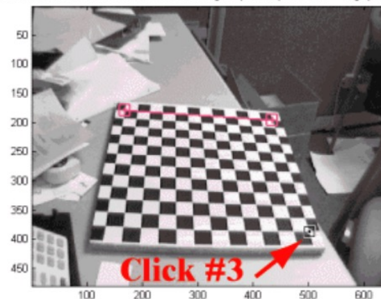
Click on the four extreme corners of the rectangular pattern (first corner = origin)... Image 1
